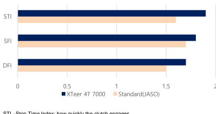
STI -Stop Time Index: how quickly the clutch engages
